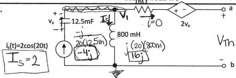
Draw a frequency-domain equivalent of the above circuit. Show a numerical phasor value for  $i_s(t)$ , and show numerical impedance values for R, L, and C. Label the dependent source appropriately.
