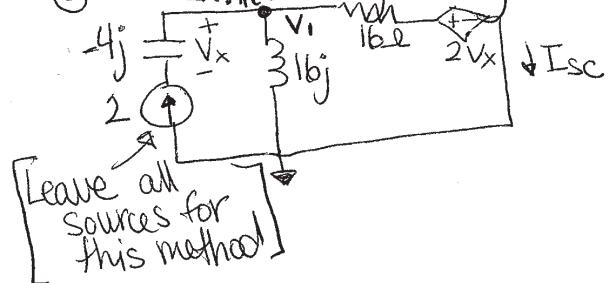
$$-2 + \frac{V_1}{16j} + \frac{V_1 - 2V_x}{16} = 0$$
