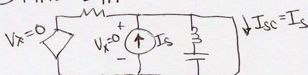
$$Z_{Th} = \frac{V_{Th}}{I_{Sc}} = \frac{2e^{j90^\circ}}{\sqrt{2}me^{-j45^\circ}}$$
