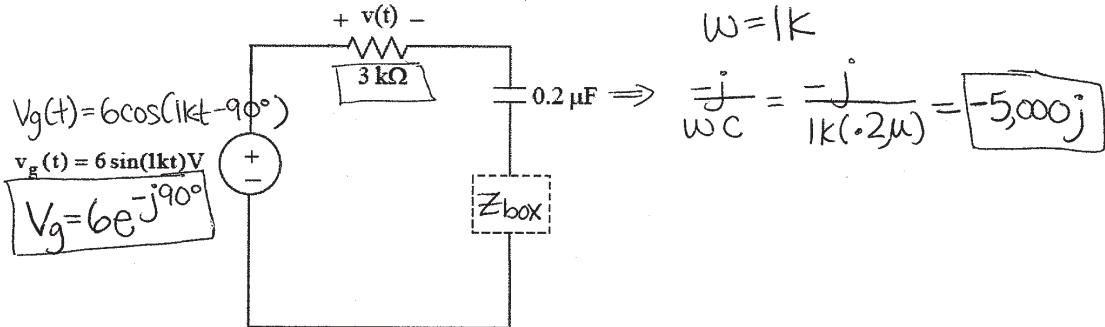
Choose an R, an L, or a C to be placed in the dashed-line box to make  $v(t) = V_0 \cos(1kt - 45^\circ)$
