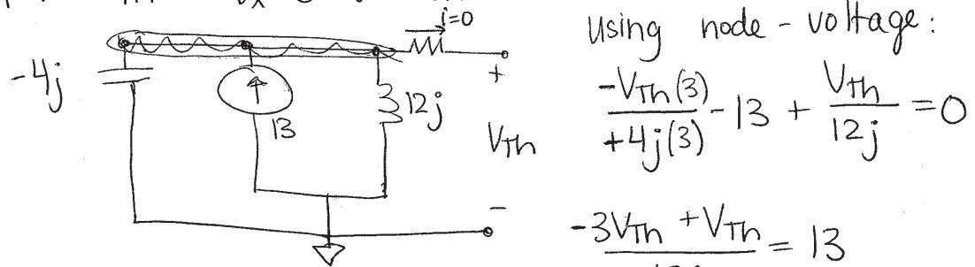
$$V_{Th}(-2) = \frac{13(12j)}{-2} \Rightarrow V_{Th} = -78j = +78e^{-j90^\circ}$$
