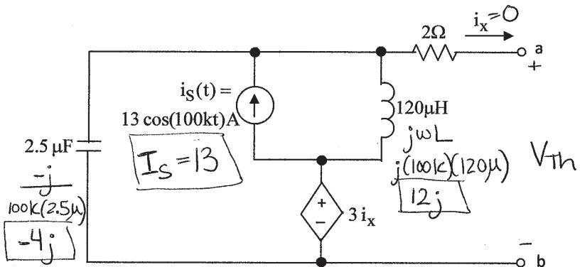
Draw a frequency-domain equivalent of the above circuit. Show a numerical phasor value for  $i_s(t)$ , and show numerical impedance values for R, L, and C. Label the dependent source appropriately.
