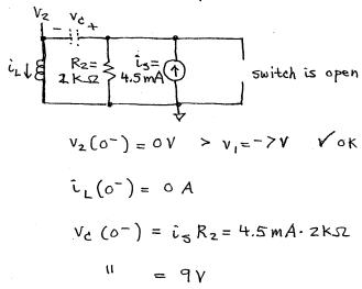
At  $t=0^+$ , we have  $i_L(0^+)=i_L(0^-)=0A$  and  $V_c(0^+)=V_c(0^-)=9V$ , whereas the voltage on the right side of the C will be OV owing to the now-closed switch.  $i_{sz}$  and  $R_z$  are bypassed.
