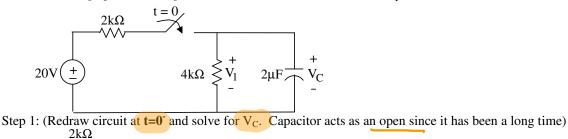
$20V \stackrel{+}{=} 4k\Omega \stackrel{+}{\leq} V_1 \stackrel{+}{=} V_C$
