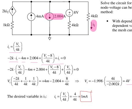
Solve the circuit for  $i_1$ . Mesh currents or node-voltage can be used. Node-voltage
