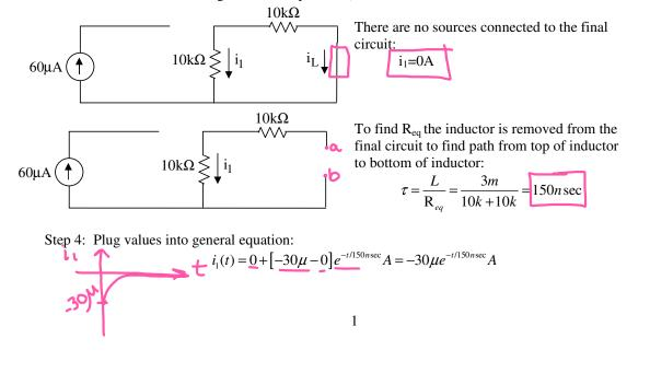
2. After being open for a long time, the switch closes at t = 0. Find  $V_1(t)$  for t > 0.
