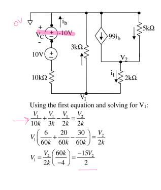
Using node-voltage to solve this circuit to find  $i_1$ : First find dependent variable in terms of nodevoltage variable,  $V_1$ .
