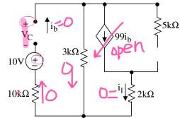
Solving for the dependent variable: ib=0 which opens the dependent source => 99ib=0 Taking a V-loop to get V<sub>c</sub> value(Be Careful-It is **not** 0 when there is a path with a V src.)  $+0+10+V_c-0=0 \implies V_c = -10V$
