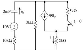
Step 1: (Redraw circuit at t=0 and solve for  $V_c$ . Capacitor acts as an open since it has been a long time)
