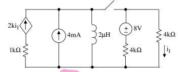
Step 1: (Redraw circuit at t=0<sup>-</sup> and solve for i<sub>L</sub>. Inductor acts as a wire since it has sat for a long time)
