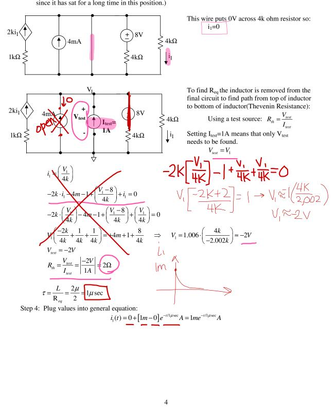
4. After being open for a long time, the switch closes at t = 0. Find  $i_1(t)$  for t > 0.
