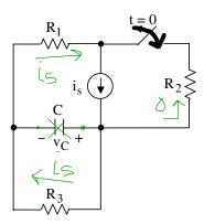
SOL'N: a) We first find the voltage across the capacitor for  $t = 0^-$ . The switch is open, eliminating  $R_2$  from consideration. The capacitor looks like an open. This leaves only the  $i_s$  source driving  $R_1$  and  $R_3$  in series. The capacitor is directly across  $R_3$  and so has the same voltage as  $R_3$ :
