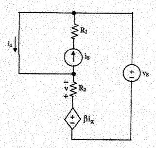
Using superposition, derive an expression for v that contains no circuit quantities other than  $i_s$ ,  $v_S$ ,  $R_1$ ,  $R_2$ , and  $\beta$ . Note:  $\beta > 0$ .
