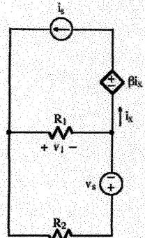
Using superposition, derive an expression for  $v_1$  that contains no circuit quantities other than  $i_S$ ,  $v_S$ ,  $R_1$ ,  $R_2$ , and  $\beta$ , where  $\beta > 0$ .
