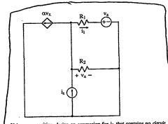
Using superposition, derive an expression for  $i_1$  that contains no circuit quantities other than  $i_5, v_5, R_1, R_2$ , and  $\alpha$ , where  $\alpha > 0$ .
