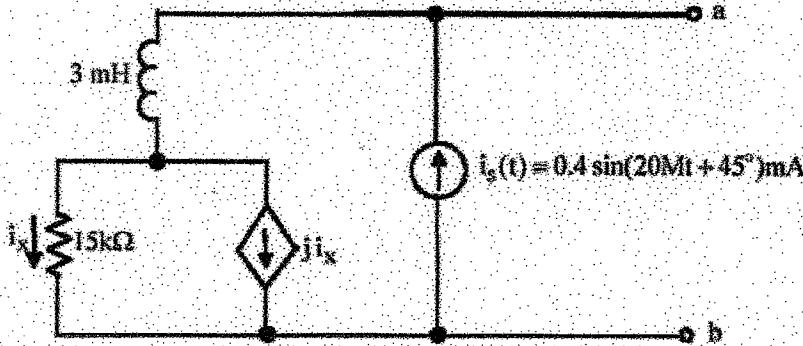
Find the Thevenin equivalent (in the frequency domain) for the above circuit. Give the numerical phasor value for  $V_{Th}$  and the numerical impedance value of  $Z_{Th}$ .
