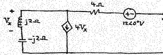
b)  $V_{Th} = V_{a,b}$  with no load.
