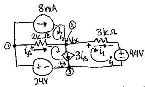
$$\textcircled{1} \quad i_p = i_3 - i_2 \quad \text{where } i_2 = 8 \text{ mA}$$
