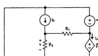
Using superposition, derive an expression for  $v$  that contains no circuit quantities other than  $i_S, v_S, R_1, R_2$ , and  $\beta$ , where  $\beta > 0$ .
