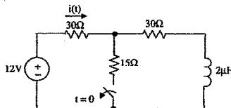
After being closed for a long time, the switch is opened at  $t = 0$ .
