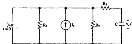
After being open for a long time, the switch is closed at  $t = 0$ .
