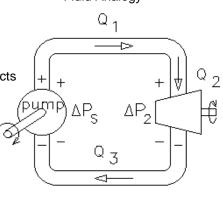
Fluids: All pressure differences are due to pumps and current flows. Pressures require no time to "move" throughout the system. Other pressure differences would equalize at the speed of sound in the fluid, which would be  $\infty$  in an incompressible fluid.
