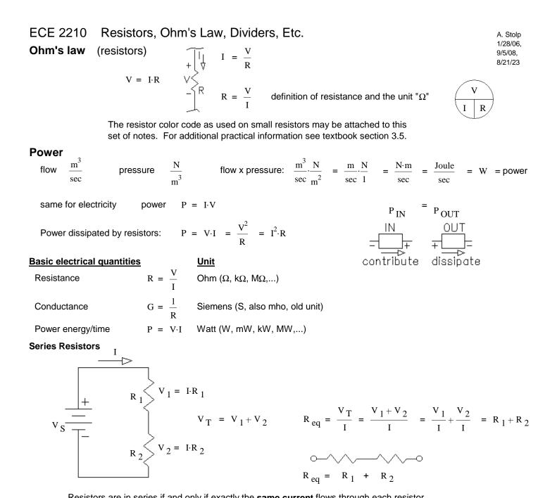
Resistors are in series if and only if exactly the same current flows through each resistor.
