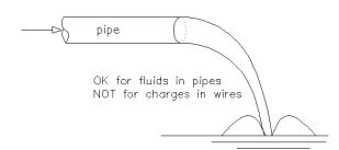
Battery also obeys KCL No accumulation of charge anywhere, so it must circulate around. Leads to the concept of a "Circuit"
