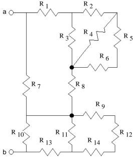
All resistor-only networks can be reduced to a single equivalent, but not always by means of series and parallel concepts.
