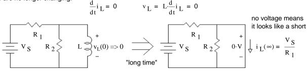
Replace the inductor with a short and find the voltage across the. Applies when sources are constant (DC)
