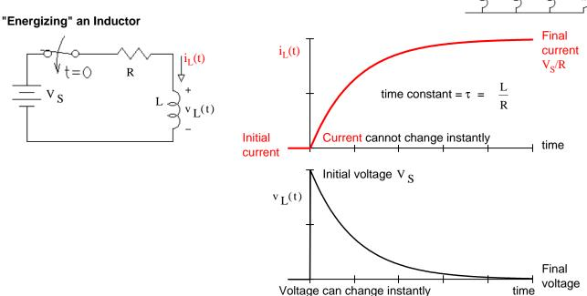
**Initial Condition** is typically found by finding the inductor current just before time t = 0.
