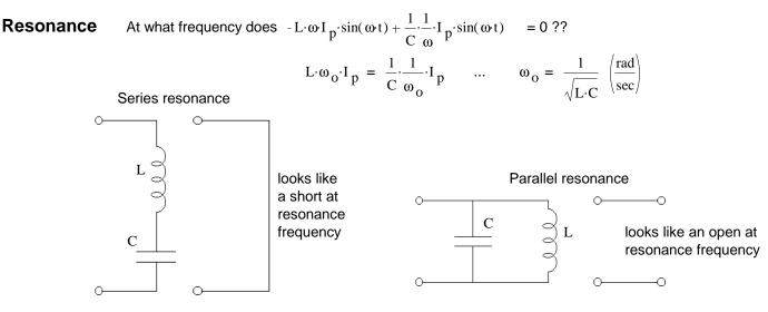
The resonance frequency is calculated the same way for either case:
