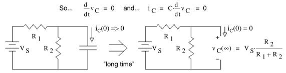
Replace the capacitor with an open and find the voltage across the open (just like finding  $v_{Th}$ ). Applies when sources are constant (DC)
