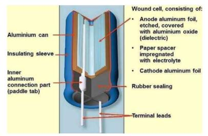
Almost all electrolytic capacitors are **polarized**. The negative terminal must always be negative with respect to the positive terminal, other wise it may be ruined.
