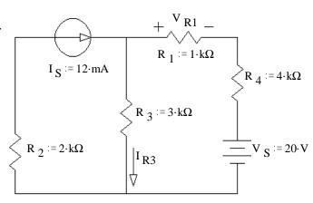
3. (23 pts) a) Find and draw the Thévenin equivalent of the circuit shown. The load resistor is  $R_{\rm L}\cdot$
