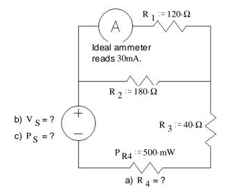
2. (20 pts) Use the method of superposition to find the voltage across R<sub>1</sub> (V<sub>R1</sub>) and the current through R<sub>3</sub> (I<sub>R3</sub>). Be sure to clearly show and circle your intermediate results.
