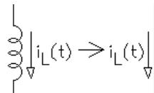
Replace inductors with wires
