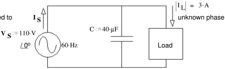
$\label{eq:power_power} \mbox{Hint 1: Since $C$ corrects the power factor, its $Q$ must exactly cancel the load's $Q$ and the source provides only $P$ and no $Q$.}$
