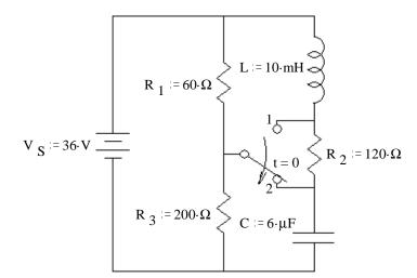
b) Find the initial condition and initial slope of  $i_L$  that you would need to have in order to find all the constants in  $i_{\rm I}(t)$ . Don't find  $i_{\rm L}(t)$  or it's constants, just the initial conditions.
