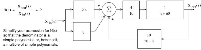
b) Find the value of K to make the transfer function critically damped.
