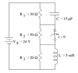
b) Find the initial condition and initial slope of  $i_L$  that you would need to have in order to find all the constants in  $i_L(t)$ . Don't find  $i_L(t)$  or it's constants, just the initial conditions.
