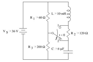
b) Find the initial condition and initial slope of  $i_L$  that you would need to have in order to find all the constants in  $i_L(t)$ . Don't find  $i_L(t)$  or it's constants, just the initial conditions.
