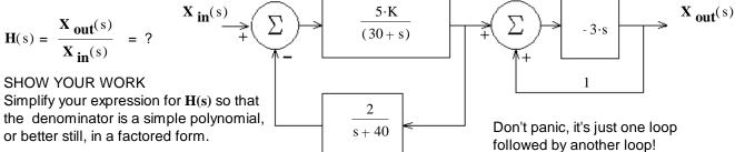
b) Find the value of K to make the transfer function of the first loop critically damped.
