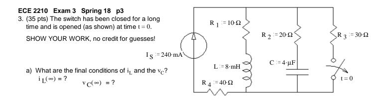
b) Find the initial condition and initial slope of  $i_L$  that you would need to have in order to find all the constants in  $i_L(t)$ . Don't find  $i_L(t)$  or it's constants, just the initial conditions.
