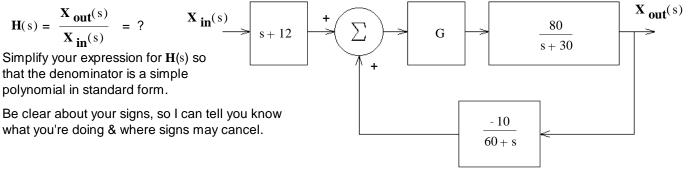
b) Find the value of G to make the transfer function critically damped.
