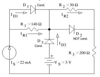
b) Based on the numbers above, was the assumption about  $D_1$  correct? yes no (circle one) How do you know? (Specifically show a value which is or is not within a correct range.)
