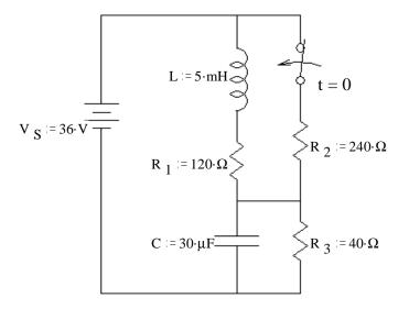
b) Find the initial condition and initial slope of  $i_L$  that you would need to have in order to find all the constants in  $i_L(t)$ . Don't find  $i_L(t)$  or it's constants, just the initial conditions.
