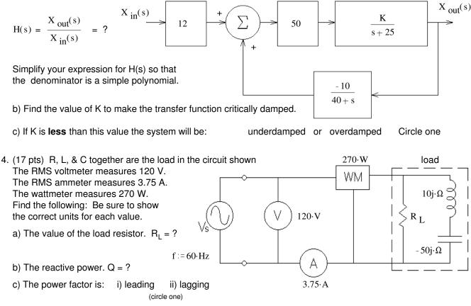
d) The 3 components of the load are in a box which cannot be opened. Add (draw it) another component to the circuit above which can correct the power factor (make pf = 1). Show the correct component in the correct place and <u>find its value</u>. This component should not affect the real power consumption of the load.
