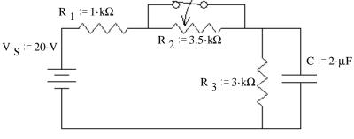
4. (14 pts) a) Find the s-type transfer function of the circuit shown.
