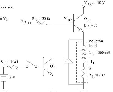
b) Find the power dissipated in transistor  $Q_2$  with this  $V_2$ .  $P_{02} = ?$
