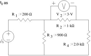
2. (14 pts) Use the method of superposition to find the current through  $R_1$ . Be sure to clearly show and **circle** your intermediate results.
