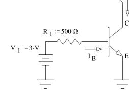
b)  $\beta = 40$  find the maximum value of R<sub>1</sub>, so that the transistor will be in saturation.
