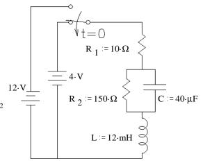
$$1 i_L(0) = 75 \cdot \text{mA} \quad v_C(0) = 11.25 \cdot \text{V}$$
