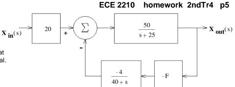
b) Find the maximum value of F so that the system does not become underdamped.
