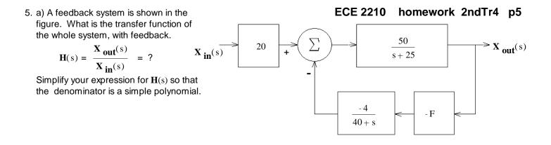
b) Find the maximum value of F so that the system does not become underdamped.
