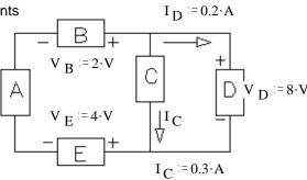
a) Which of the components are absorbing power from the circuit?
