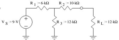
b) Find the voltage across  $R_L$  (  $V_L$ ) and the current through  $R_L$  ( $I_L$ ) using your Thevenin equivalent circuit.
