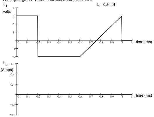
4. The voltage across a 0.5 mH inductor is shown below. Make an accurate drawing of the inductor current. Label your graph. Assume the initial current is 0 mA.
