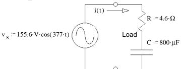
b) Compute the average power dissipated by the load.
