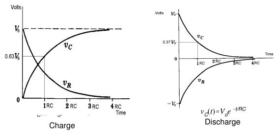
Where  $v_c(t)$  is the capacitor voltage as a function of time,  $V_s$  is the source voltage during charging (The Thévenin voltage for us), and  $V_o$  is the initial voltage across the capacitor at the time that discharge begins.
