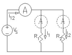
Record the ammeter reading  $(I_{12})$ . Move the ammeter into the two other positions shown by the dotted outlines in the drawing above and record all the currents  $I_1$  and  $I_2$ .
