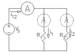
Since current must flow through the ammeter for it to work, you will need to do some rewiring each time you move the ammeter (See box on previous page). Admittedly, this is a pain in the neck but it is good practice. Be very careful with your wiring.
