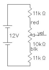
Measure the voltage between the two outside leads of the "Input Position" pot. Turn the pot through its range. Does this voltage change significantly? Now measure from the black to the yellow lead and try it again. What range of voltages do you measure?
