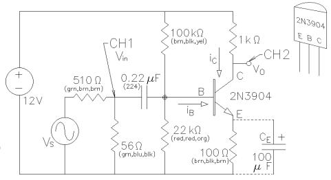
Please note that the 510  $\Omega$  and 56  $\Omega$  resistors are NOT part of the amplifier. They are needed because the function generator output  $(V_{pp})$  cannot be turned down low enough for this circuit. Together they constitute a voltage divider which reduces  $v_s$  by about a factor of 10. The actual  $v_{in}$  of the amplifier circuit is measured where CH1 is connected.
