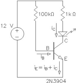
whereas the collector current flows through only a 1 k $\Omega$  resistor. The base current (the controller) is roughly 1% of the collector current (which it controls)! A very small current controls a much larger current.
