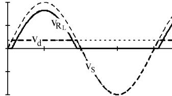
Place a 47 to 220 µF capacitor in parallel with the load resistor (remember the capacitor polarity—you don't want to blow up the capacitor). Observe and sketch the filtering effect of the capacitor. The load voltage is better than it was, but it's still not great. The DC voltage still has significant "ripple". Measure the peak-to-peak voltage of this ripple. Add a second capacitor in parallel with the first. Comment about how the added capacitance effects the ripple.
