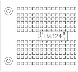
Most op-amp circuits won't work right unless the op-amp is powered with both + and - power supplies. This can be inconvenient, but using op-amps with single-sided supplies is tricky. REMEMBER this! One common mistake people make with op-amps is trying to use them with a single power supply.
