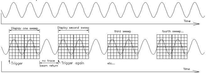
The second shows the pieces that will be seen on the scope screen. In this example the scope is triggering at 0V and a + slope. Why does it need to differentiate between + and - slope to get a stable trace? Explain triggering in you notebook in your own words.
