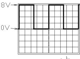
Observe the transient. Does it look like an exponential curve? Does the capacitor voltage ever change from one value to another instantaneously? Draw this transient ( $v_c$ ) in your lab notebook. Make the vertical axis range of your drawing at least -8 V to +8 V so you can add a drawing of the resistor transient ( $v_p$ ) later.
