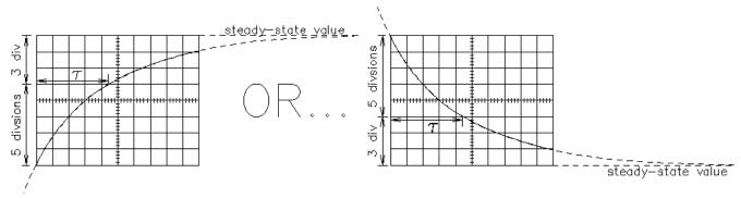
Readjust the scope to see the entire charge or discharge curve like you sketched before you took the time constant measurement. Now swap the positions of the resistor and capacitor. Sketch this new transient  $(v_R)$  on your previous sketch. If you added these two traces at each
