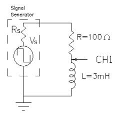
voltage change instantaneously, in the inductor it's the current which shouldn't change instantaneously.
