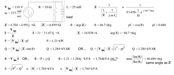
OR, since we know that the voltage across each element of the load is  $\rm V_{in}$  ... Real power is dissipated only by resistors
