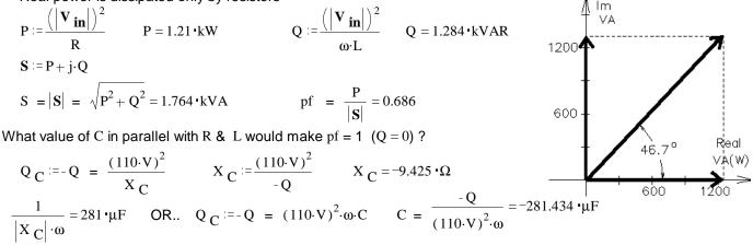
**Ex. 2** R & L together are the load. Find the real power P, the reactive power Q, the complex power S, the apparent power |S|, & the power factor pf. Draw phasor diagram for the power.
