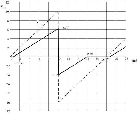
A voltage waveform (dotted line) is applied to the circuit shown.  $\underline{\text{Accurately}} \text{ draw the output waveform } (v_o) \text{ you expect to see}.$ Label important times and voltage levels.
