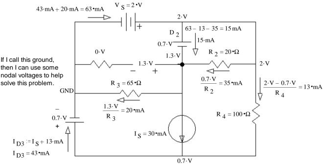
Alternate way to find:  $I_{D2} = 20 \cdot \text{mA} + I_S - \frac{0.7 \cdot \text{V}}{R_2}$   $I_{D2} = 15 \cdot \text{mA}$
