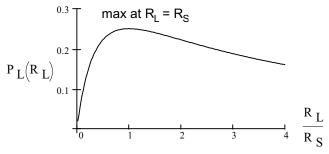
This is rarely important in power circuitry, where there should be plenty of power and  $F_{\rm S}$  should be small. It is much more likely to be important in signal circuitry where the voltages can be very small and the source resistance may be significant -- say a microphone or a radio antenna.
