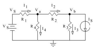
Write the KCL equations at each unknown node:
