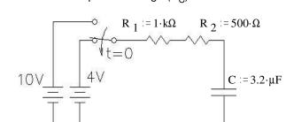
4. The switch below has been in the upper position for a long time and is switched down at time t = 0. At what time is  $v_C = 4 \text{ V}$ ?
