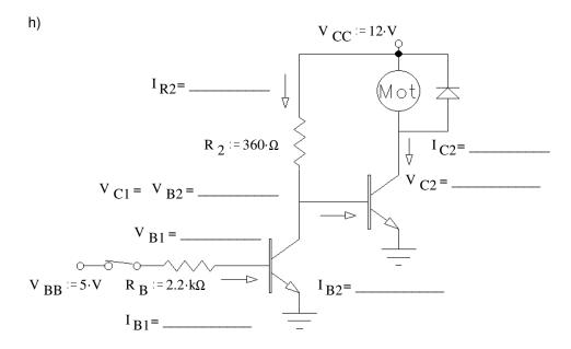
2. In problem 1b, What is the largest value that  $R_B$  could be and still keep the transistor in saturation?
