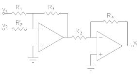
6.) Draw a differential amplifier. Choose an  $R_{in}$  value. Make  $R_f$  12 times bigger than  $R_{in}.$  Say  $R_{in}$  = 10 k $\Omega$  and  $R_f$  = 120 k $\Omega.$
