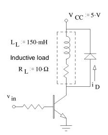
b) If the diode ever conducts, what is the maximum diode current you expect.
