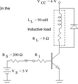
b)  $\beta = 80$  find the maximum value of  $R_1$ , so that the transistor will be in saturation.
