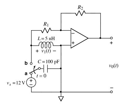
After being in position **a** for a long time, the switch moves to position **b** at time t = 0.
