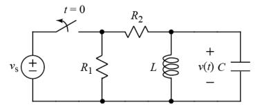
After being closed for a long time, the switch opens at t = 0. L = 10 nH C = 250 nF  $R_1 = 0.1 \Omega$   $R_2 = 0.025 \Omega$ If  $v_s = 10 \text{ V}$ , find v(t) for t > 0.
