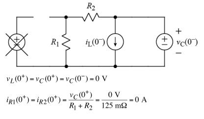
No current flows through the R's, so all the current in the L must flow through the C (but in the negative direction, since we are measuring currents in the down direction):
