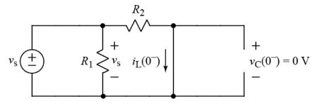
The L, acting like a wire, shorts out the C. Thus, the initial C voltage is zero:
