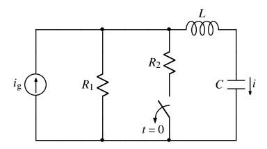
After being closed for a long time, the switch opens at t = 0.
