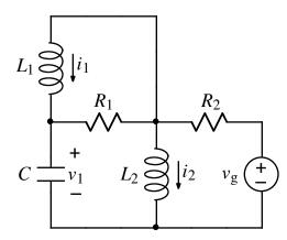
At t = 0,  $v_g(t)$  switches instantly from  $-v_o$  to  $v_o$ .
