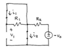
$i_1(o^-)=0$  since there is open circuit at  $v_1$  and  $R_1$  is shorted, (so no current in any direction from node on left side of  $R_1$ ).
