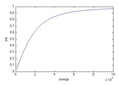
c) We find the cutoff frequency by setting the magnitude of the transfer function equal to  $1/\sqrt{2}$  times the max value of |H|.
