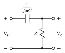
The voltage-divider formula gives the transfer function, starting with the formula for  $V_o$ :
