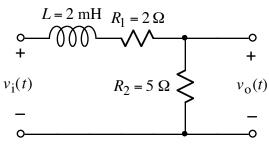
For the above circuit, determine the transfer function  $H(j\omega) = V_o/V_i$ .
