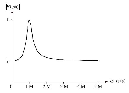
Given the resistor connected as shown and using not more than one each R, L, and C in the dashed-line box, design a circuit to go in the dashed-line box that will produce the **band-pass**  $|H(j\omega)|$  vs.  $\omega$  shown above. That is:
